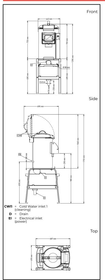
Electric Supply voltage: 603515 (DT15E1C) 220-240 V/1N ph/50/60 Hz 200-240/380-440 V/3 603516 (DT15E324C) ph/50/60 Hz Electrical power max: 0.37 kW 0.37 kW **Total Watts:** Capacity: Performance (up to): 240 kg/hour Capacity: 15 litres Key Information: External dimensions, Width: 440 mm External dimensions, 690 mm Depth: External dimensions, Height: 750 mm
